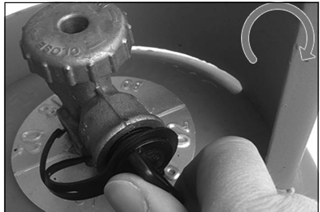
3. Check the bullnose connection on the regulator for any visible damage before connecting to the cylinder.
